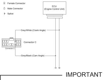
If the Crank and Cam angle signal wires are connected to the ecu, e-manage will recognize the rpm without connecting the rpm signal wire.
