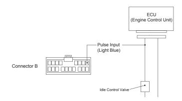
\* When using the Idle Adjustment Setting, make sure to set the Jumper JP16 to "OPEN" in the unit
