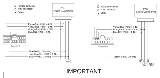
On a vehicles with low resistance injectors without dropping resistors (AE86, R31), change the injectors to high resistance injectors or add a dropping resistors.
