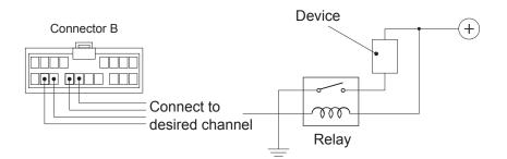
•When using this feature the proper channels must be configured in the "I/J" set up in the Parameter setting in the software and make the necessary jumper setting to activate these channels.
