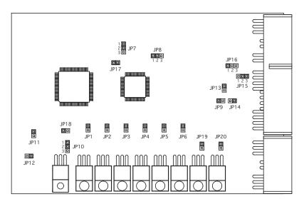
When Jumping "1-2" or "2-3" make sure to match the pin numbers printed on the circuit board at the coresponding jumper locations.
